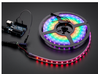
Figure 2: NeoPixel LED strip (60 pixels)
