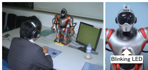
Fig. 3. Experimental environment and robot with embedded LED
